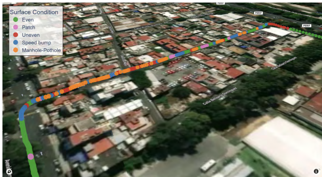
Figure 8. Spatial mapping of continuous anomalies along a severely degraded route section.
