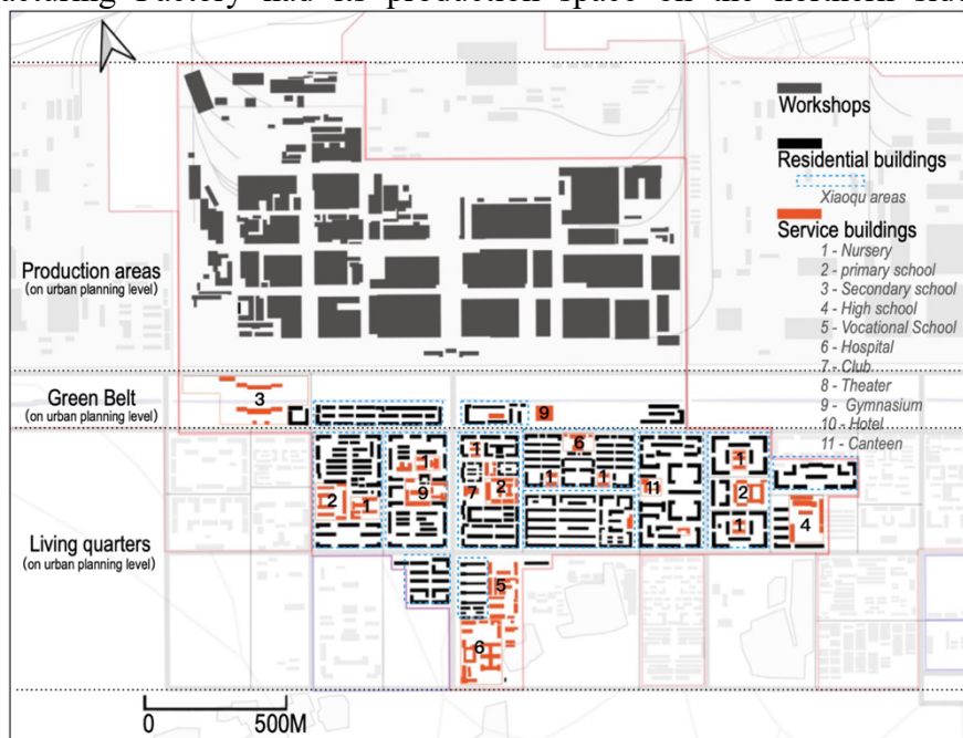
Fig. 6-10 The spatial structure of large scale danwei, use the No.1 tractor factory as an example
