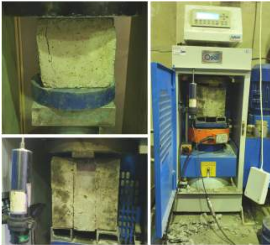
Fig. 5. Mechanical testing setups for compressive and shear-splitting tests.
