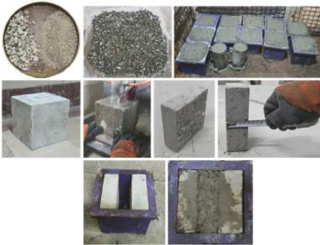
Fig. 4. Fabrication process of composite specimens.
