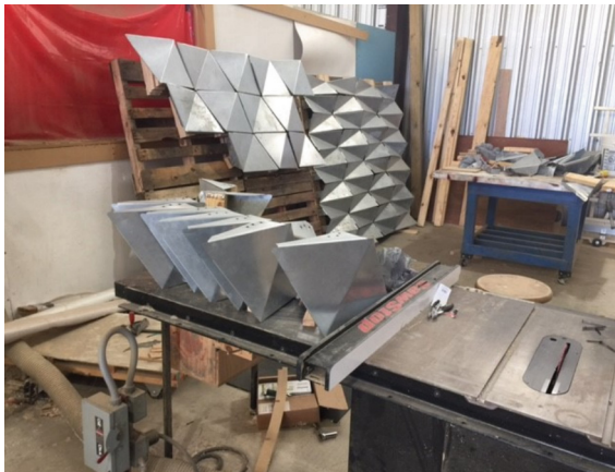
Fig. 5. (photo) 2022 Fabrication and assembly of multiple metal façade units using real galvanized Sheetmetal by students (Photograph by the Author).
