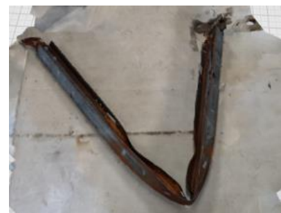
Figure 1(b). Deformed steel post
