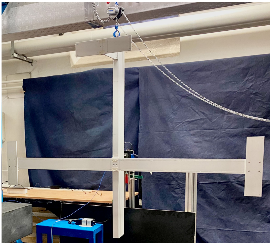
FIGURE 1 Garteau laboratory-scale model and fibre-optic arrangement in the test configuration. The shaker is connected to the rear part of the fuselage, and the suspension system is located in the upper part.
