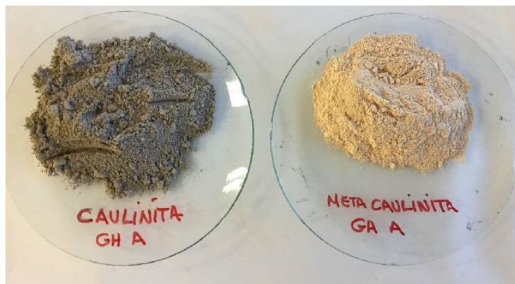
Fig. 7: Preparation of the metakaolin sample. a) Muffle kiln, b) comparison of the sample before (kaolin) and after the calcination (metakaolin).
