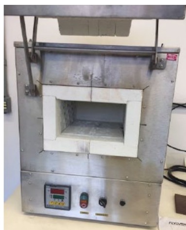
Fig. 7: Preparation of the metakaolin sample. a) Muffle kiln, b) comparison of the sample before (kaolin) and after the calcination (metakaolin).
