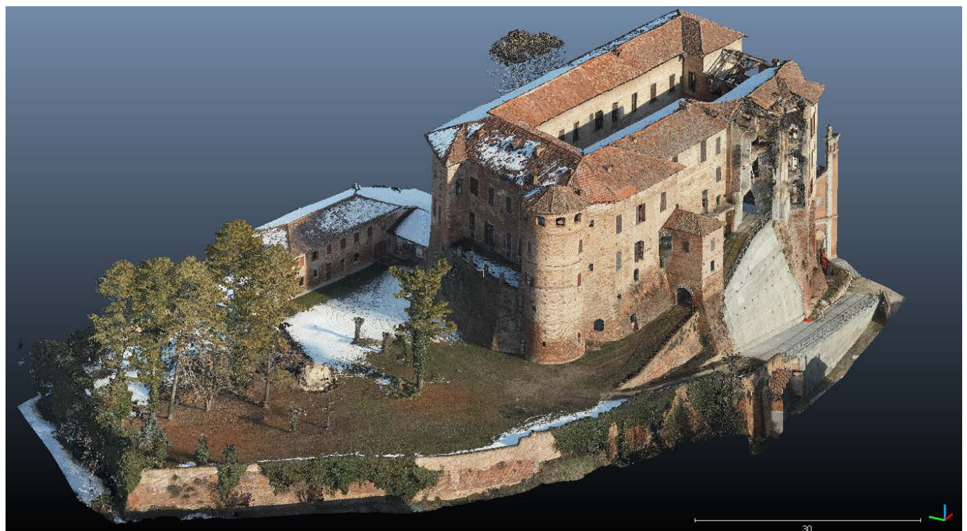
Figure 7. Photogrammetric clouds of the entire castle and surroundings (point dimension 1 pixel).
