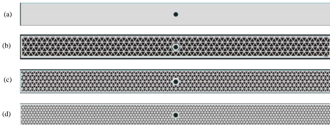
Fig. 6 (a) solid beam, (b) infill percentage of 28%, (c) infill percentage of 37%, (d) infill percentage of 55%
