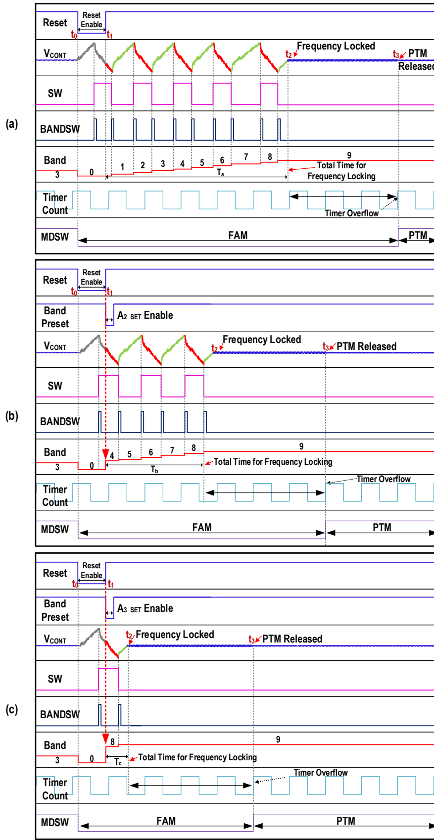
Fig. 17. Critical transient waveforms of our HCC with band preset signal enabled.
