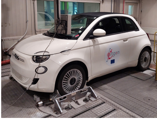
Figure 16: Electric vehicle used to carry out the verification of the proposed control approach under standardized driving cycles.
