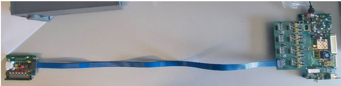
(c) A TIMESPOT1 connected to the mezzanine with a 1 m long cable.
