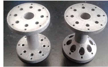
Fig. 11 AlSi10Mg prototypes of Ka-band circular waveguides manufactured through SLM.
