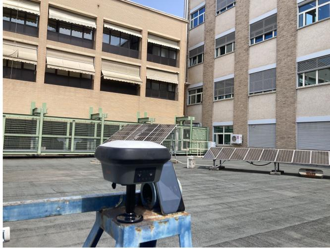
**Figure 2:** GNSS data collection scenarios with intensive multipath/NLoS.
