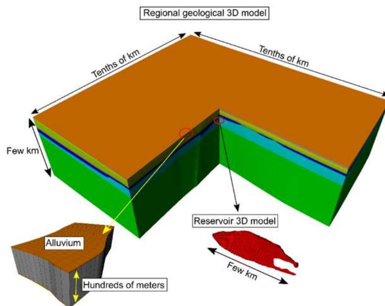
**Figure 8.** 3D view of the regional geological and reservoir models used for land settlement analysis during geomechanical simulations and for flow simulations, respectively (figure modified from [21]).
