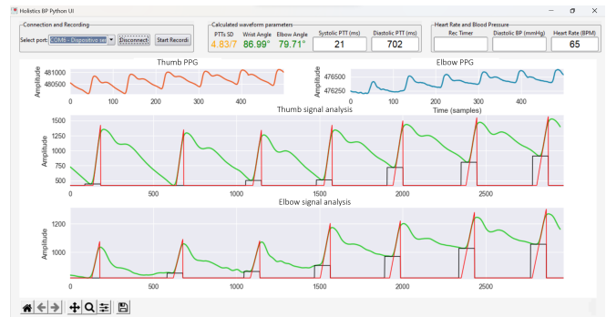
Fig. 3. Graphic User Interface used by the device in the blood pressure assessment. The upper plots show the thumb signal (red) and elbow signal (blue). Bottom plots depict the intersecting tangent being extracted from gathered signals for PTT estimation.
