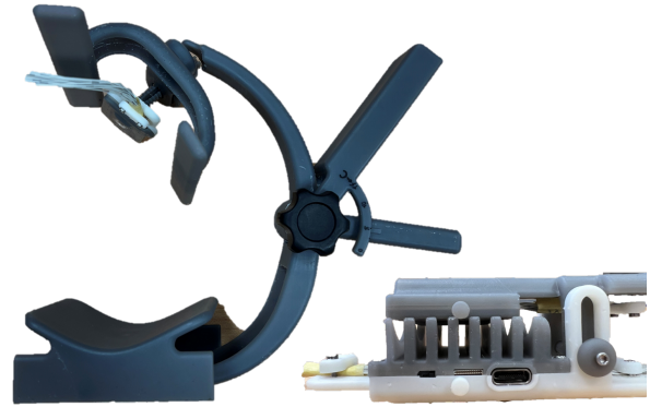
Fig. 2. 3D printed enclosures realized for the blood pressure device. Support containing the elbow's sensor (left). Finger clip holding the thumb sensor (right).
