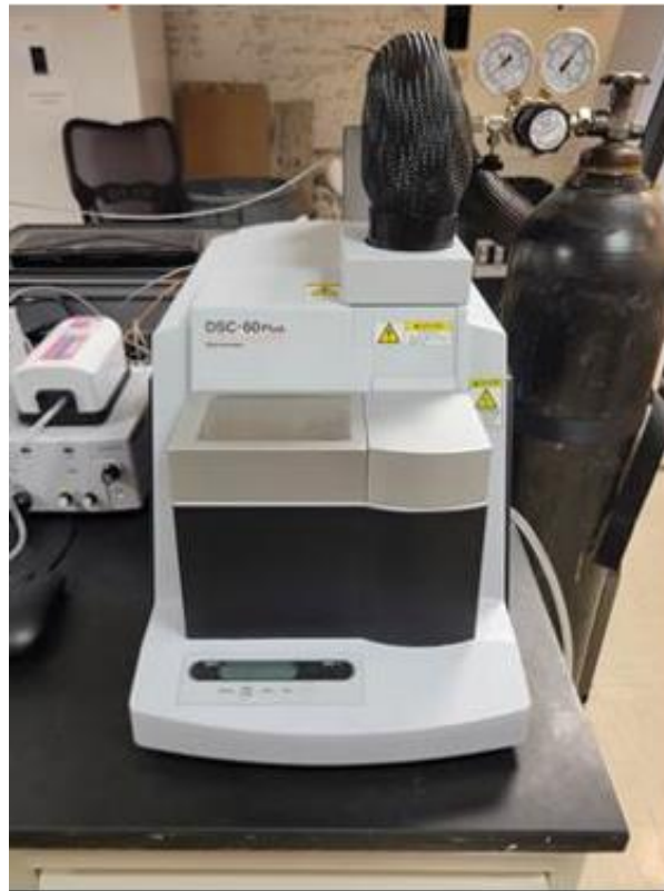
Figure 29. Test setup showing DSC in operation
