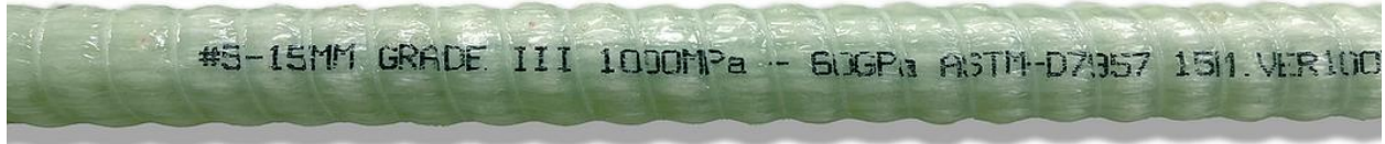
Figure 24. FRP bar manufactured by MST
