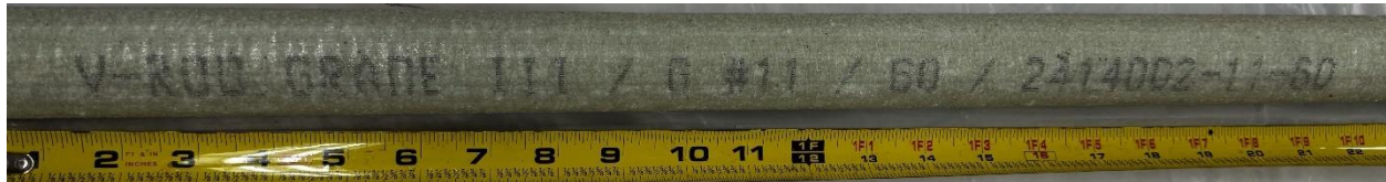
Figure 25. FRP straight bar #11 manufactured by Pultrall.
