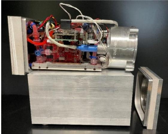
**Figure 2. AIM experiment cube hardware**
