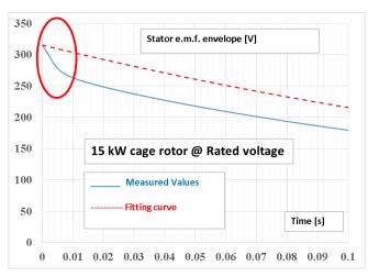
Fig. 7. Magnification of the first instants of the flux-decay test.
