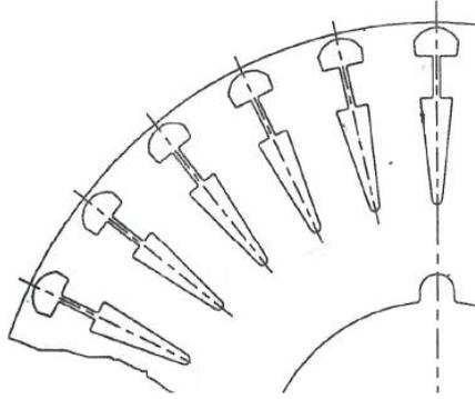
Fig. 15. Section of the rotor slots of the motor under test.
