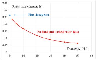
Fig. 12. Rotor time constant as a function of the frequency and comparison with the value obtained with the flux decay test.
