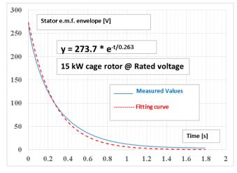
Fig. 8. Back-emf transient by neglecting the initial measurement data.
