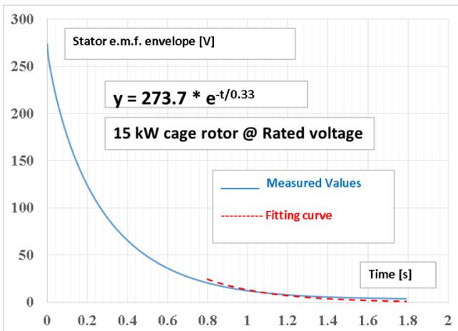
Fig. 10. Back-emf transient at the end of the flux-decay test.
