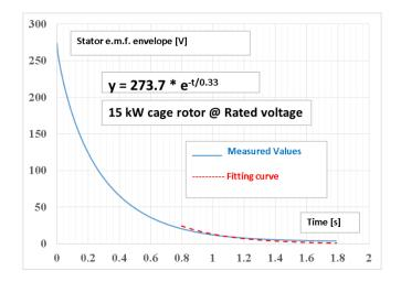
Fig. 10. Back-emf transient at the end of the flux-decay test.
