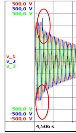
Fig. 6. Stator voltage spikes at the machine terminals.
