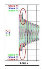
Fig. 6. Stator voltage spikes at the machine terminals.
