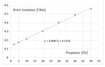
Fig. 13. Rotor resistance as a function of the frequency.
