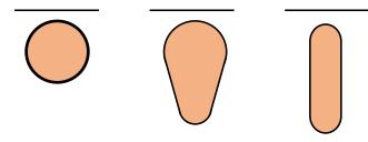
Fig. 2. Examples of closed rotor slots.
