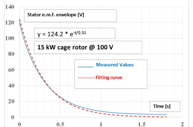
Fig. 11. Flux-decay results for a supply voltage of 100 V.
