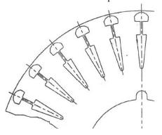
Fig. 15. Section or the rotor slots of the motor under test.
