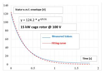
Fig. 11. Flux-decay results for a supply voltage of 100 V.
