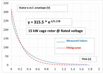
Fig. 5. Measured envelope of the back-emf and fitting curve.
