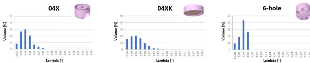
Figure 2: lambda distributions for the three different caps at 10° BTDC.
