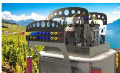
4-MF: Multi-Flanges™ allowing to test 4 cells in a same run
