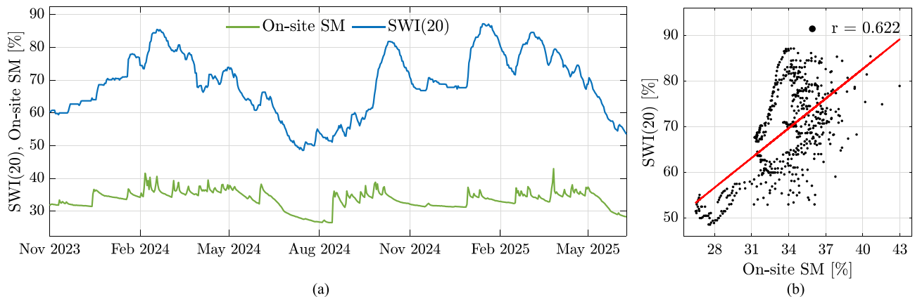
Figure 8. Correlation between SWI(20) and on-site SM: (a) overlapped time series and (b) scatter plot.
