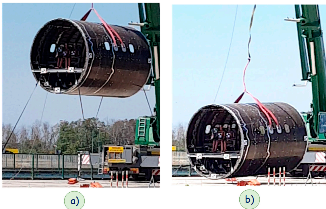
Figure 6. Fuselage section drop test: (a) Before the drop test; (b) during the fall.
