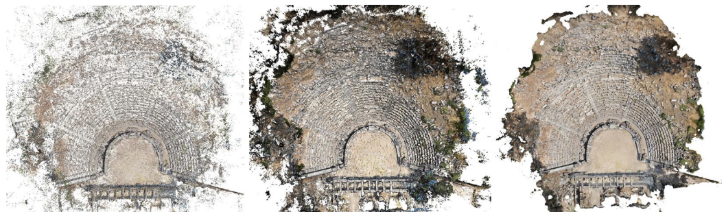
Figure 5. Images of the post-processing of data for the Theater. From the left, the alignment of cameras (1,256,561 points), dense cloud (261,238,304 points), and textured mesh (43,646,219 faces and 21,831,522 vertices). (E.C.G.).
