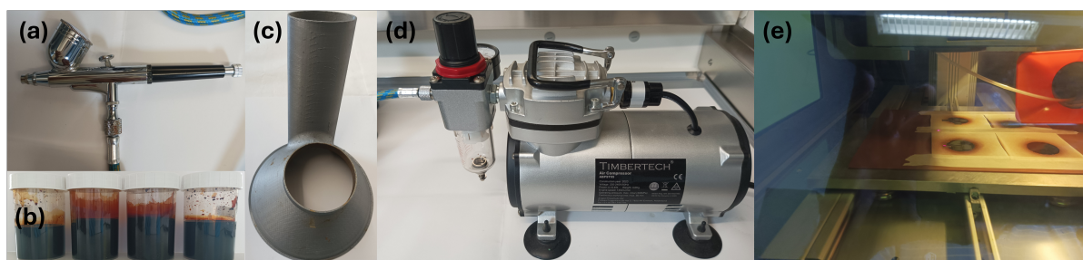
Fig. 2.7 Experimental arrangement for LIG formation on lignin-based coatings, showing the (a) air brush (b) bio polymers (c) masking system (d) air compressor, and (e) CO 2 laser etching process for formation of laser induced graphene on bio polymer coatings.
