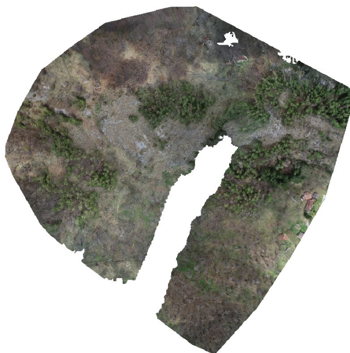
Figure 6. The orthophoto obtained considering the first set of 150 images.
