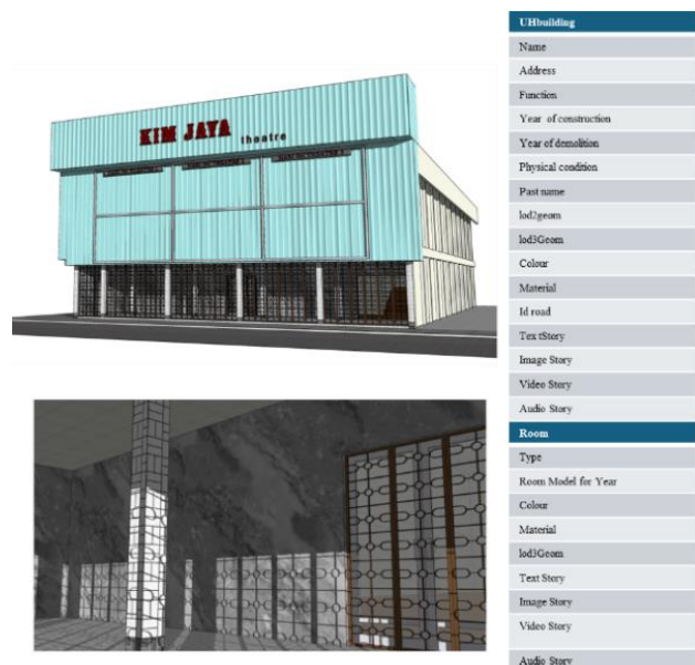
Figure 8. Example of 3D model and its semantic information.
