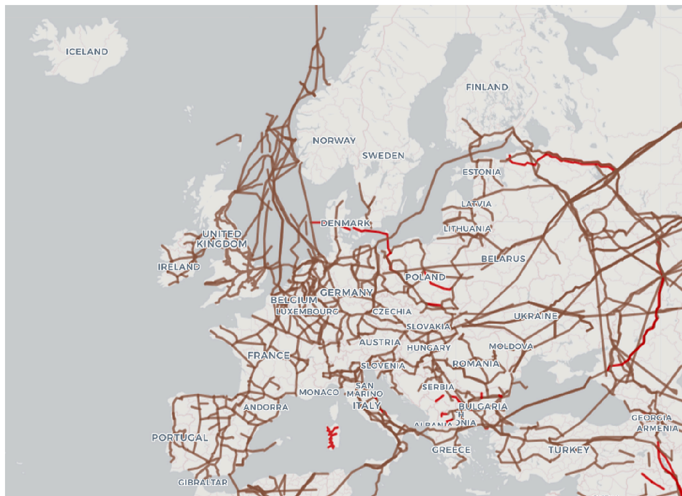
Fig. 1. 2023 EU natural gas grid in operation (brown) and under construction (red). [10]. (For interpretation of the references to colour in this figure legend, the reader is referred to the web version of this article.)
