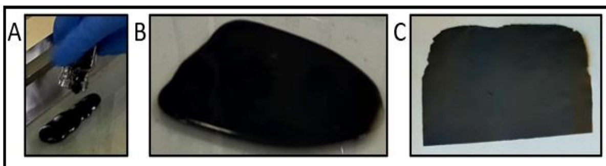
Figure 1. GO membrane slurry (A,B) and after being cast on the glass support (C).
