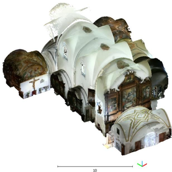
Fig. 4. Point cloud obtained by XGRIDS LIXEL L2 handheld laser scanner.
