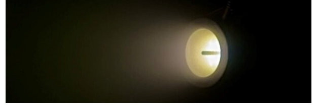
Fig. 3. Photo of ECRA thruster operated with iodine inside ONERA facility, at a volume flowrate of 1.5 sccm, 25 W of input power, at a pressure of 1.65 \cdot 10^{-5} mbar (without cryogenic system).
