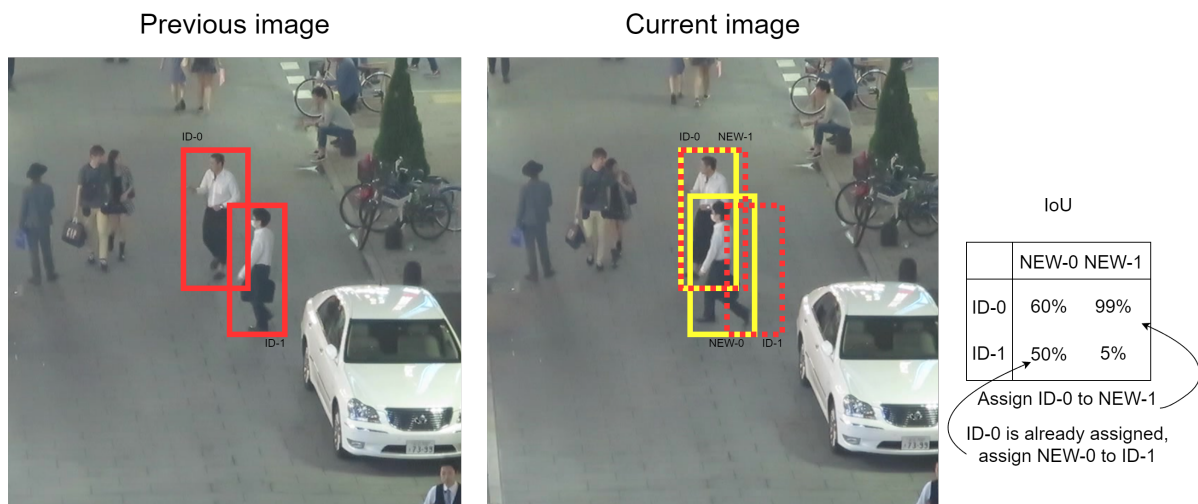
Fig. 4.2 The IDs of old detections (red) are saved in the cost matrix and assigned to the new detections (yellow) according to the IoU value, prioritizing detections with higher overlapping.
