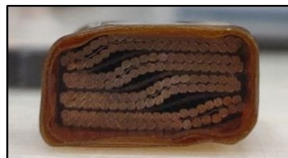
Fig. 5. Buckling failure of the first test specimen.
