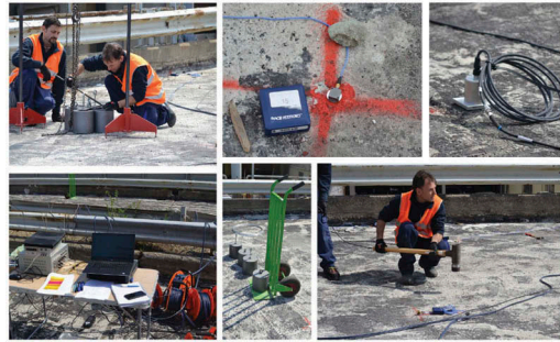
Figure 11. Dynamic identification experimental tests.
