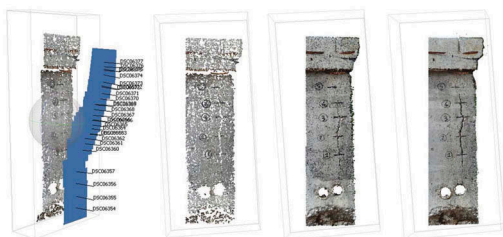
Figure 13. Mapping of photographic images to 3D surfaces.
