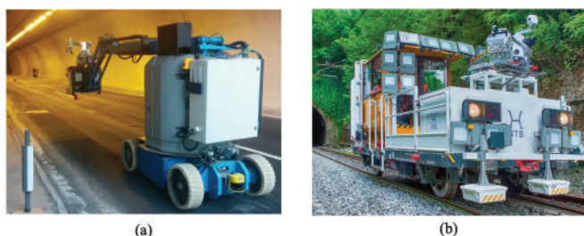
Figure 22. (a) ROBO-SPECT 77 and (b) ARCHITA 81 robotic platforms for tunnel inspection
