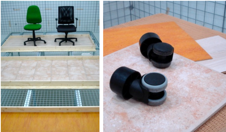
Figure 1. The materials tested in the dead room in the C1 and C2 tests are shown in the picture on the left: LLC and HLC on the left and right, respectively, in the upper part of the image; the three paved platforms, provided with the wooden flooring (at the top), the ceramic flooring (in the middle) and the PVC flooring (at the bottom), were placed on top of the floating grid. The materials (ceramic, PVC and wood floorings) tested in the dead room in C3 are shown in the picture on the right: both the LLC wheel and the HLC wheel were provided with handles.
