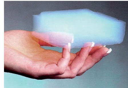
Aspetto aerogel, solido secco semitrasparente da https://nanografi.com/blog/promising-invention-in-the-insulation-industry-by-nanotechnology-aerogel/
