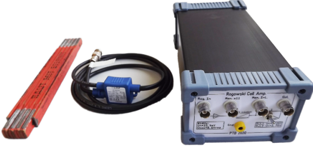
Fig. 7: Rogowski coils with the corresponding electronic integrator.
