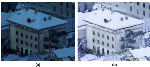
Figure 2. Radiometric information enhancement. Point cloud processed with acquired images (a) and after image correction (b).
