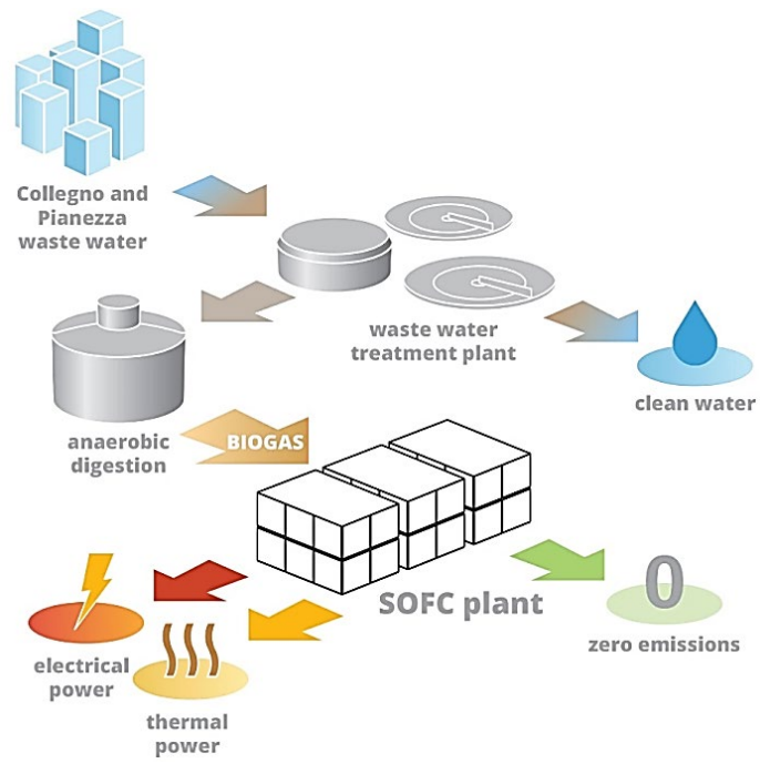
Figure 16. Concept diagram of the DEMOSOFC plant [14].
