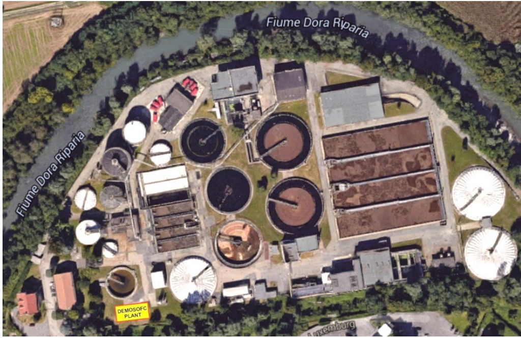
Figure 15. SMAT wastewater treatment plant in Collegno (Turin) [16]. “DEMOSOFC Plant” shows the area 798 where the three SOFC modules will be installed.
