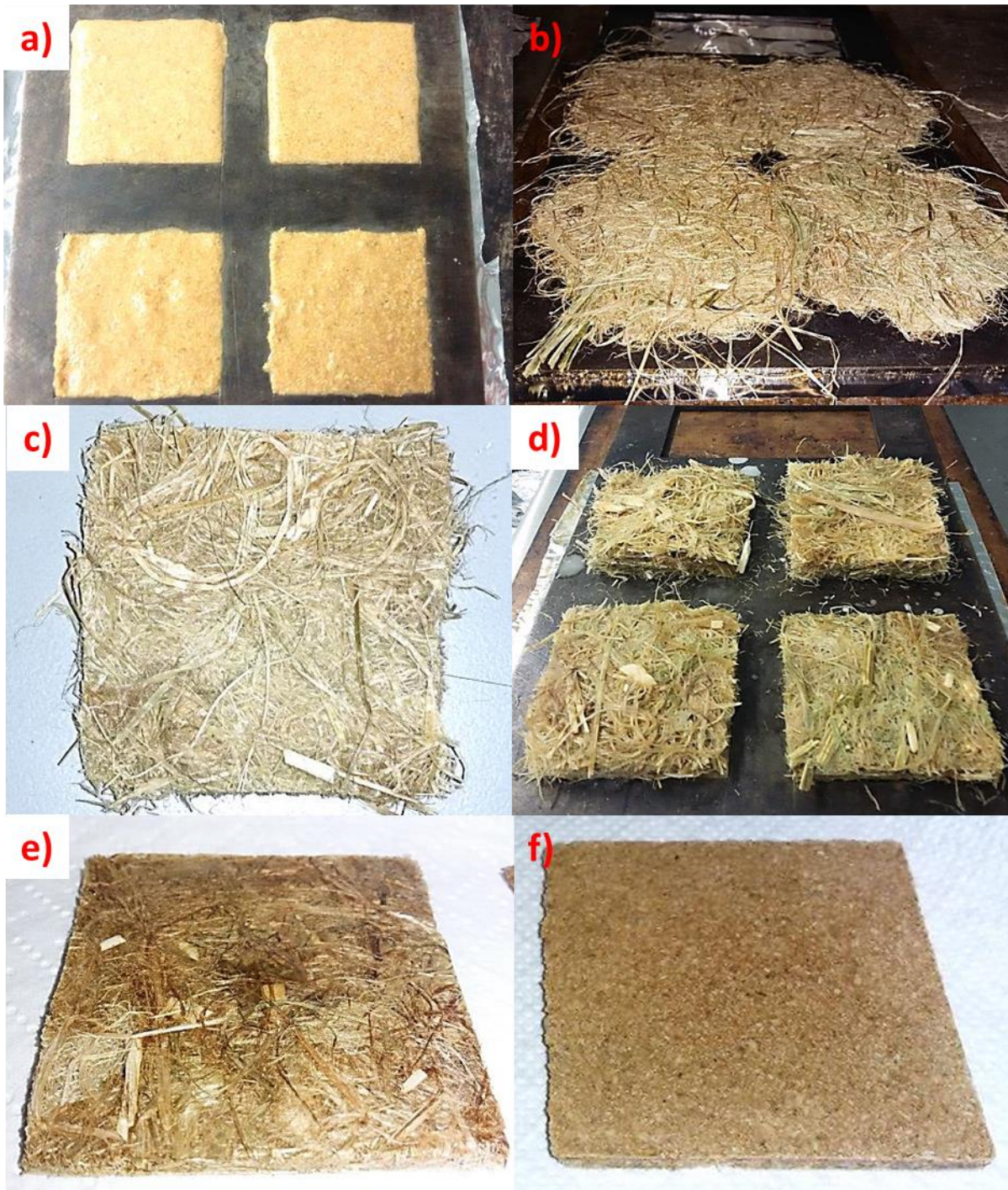
Figure 2. Photographs of slurry of water, starch and rice husk (a), pressed hemp fibers (b), cut hemp mat (c), hemp mat impregnated with water and starch (d), final specimen H-S (e) and final specimen R-S (f).
