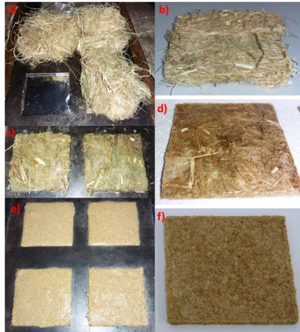
Figure 1 Digital pictures of pressed hemp fibres (a), hemp mat (b), hemp mat impregnated with water and starch (c), sample H-S (d), slurry of water, starch and rice husk (e) and sample R-S (f).
