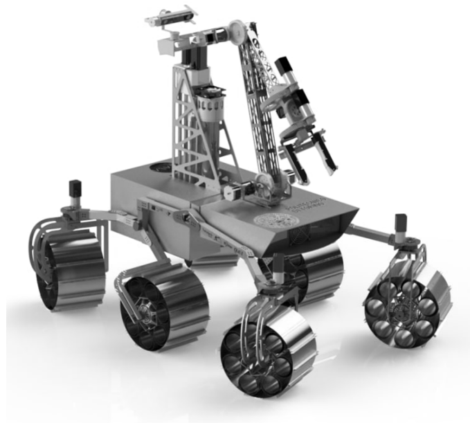
Figure 2. A 3D rendering of the Ardito Rover developed by the D.I.A.N.A. student team of Politecnico di Torino.
