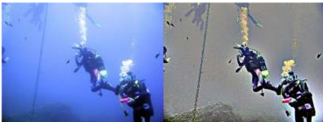
Figure 2: Original image on the left and the Low level filtered image on the right, for the parameters having the default values (Scale = 240; Scale division = 3; Dynamic slider = 1,2). (Original image from flickr, Courtesy gingio for Wikipedia).
