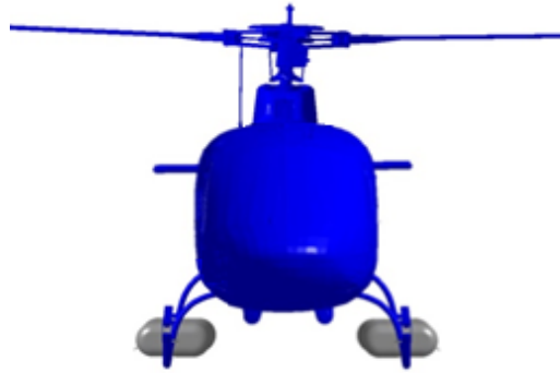
Figure 2 – Symmetrical dual basket configuration
