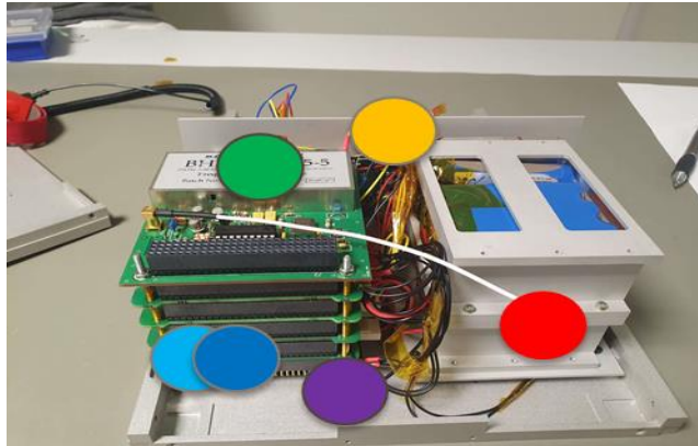
Fig. 7 Position of the Temp sensor in the Service box
