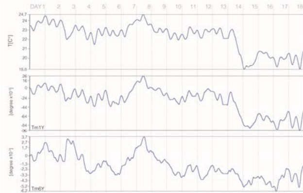
Figure 32 Data acquisition of temperature-gauge and tilt meters Tm1, Tm6 along y-direction for a time window covering major strengthening operations on the buttresses.
