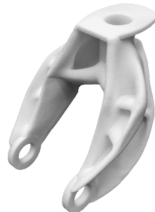
Fig. 6. Conceptual prototype realized through SLS.
