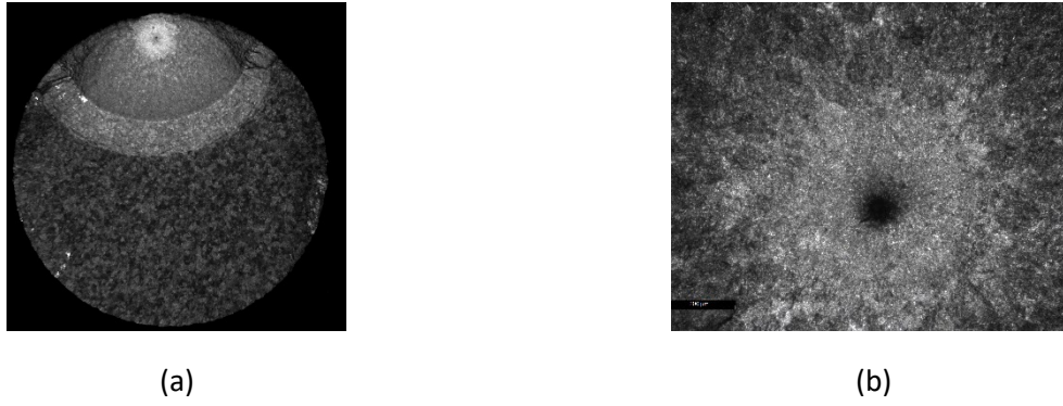
Figure 6: Fish-eye fracture found experimentally: a) fish-eye morphology; b) enlargement of the ODA.
