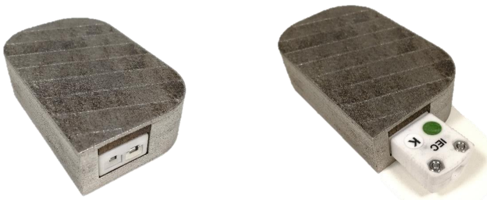
Fig. 4. Sample released in final configuration with integrated sensor and external connection.
