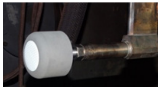
Figure 28 Stagnation test assembly.
